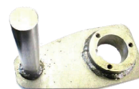
5,6. CAM ARM and SPLIT TAPER BUSHING
