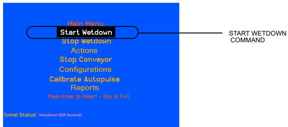
**Figure 79. Start Wetdown Command on WBC Built-in Monitor**
